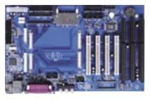
ETX-DB-7SR-R20 Full Function ETX Baseboard with LCD/CRT VGA, Audio, DOC, CF II & D I/O
