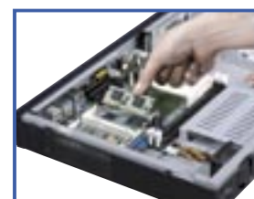
Expendable two Socket-PCI for add-on LAN module
