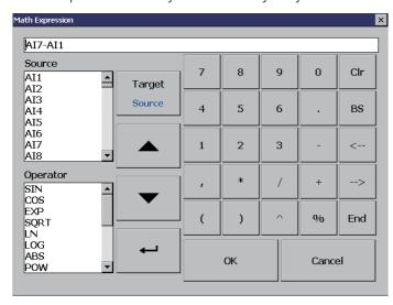
**External Channels:** Besides Al & DI inputs, PR recorders accept inputs through communication called External Channels. PR10, PR20 & PR30 can work External Channels maximum up to 24, 48 & 96 respectively.
